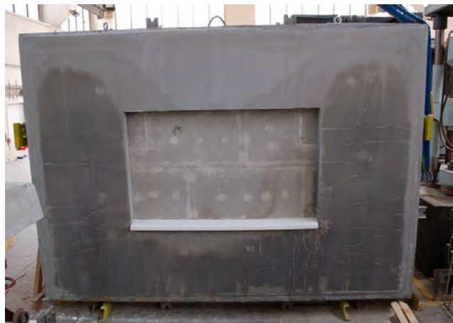
Test rig with enlarged opening after completed hygrothermal behavioural cycles according to EN 16383
